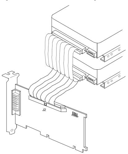
Figure 1.3 Internal SCSI Devices Chained Together
